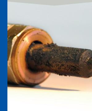
DIESEL FUEL INJECTOR AFTER TREATMENT
